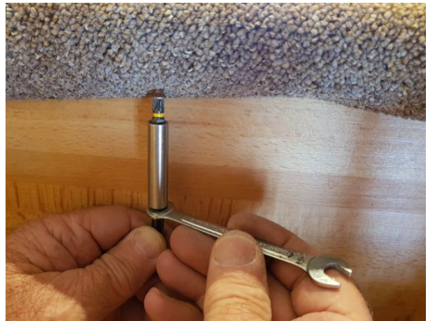
Rick's ingenious tool to fix the carpet at the top of the stairs - he wore the skin away from his fingers.
